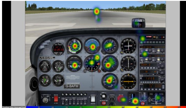
Fig. 3.4. The Heat Map option, the color of an area is depended on the fixation time, starting with blue (short duration) to red (long duration)
