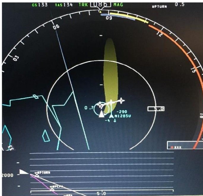
Figure 13. ND showing that a turn to the right will result in an alert
