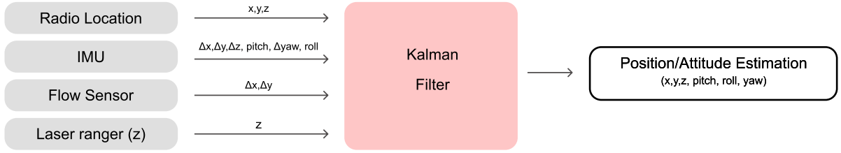
Fig. 6 Position and attitude estimation using a Kalman filter
