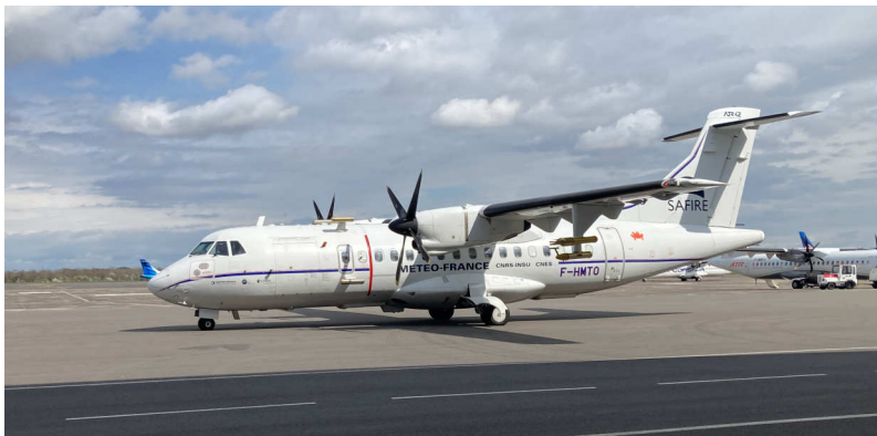
Fig. 2 Safire ATR 42-320 flight test bench (MSN 78): aircraft with all modification for the SENS4ICE European flight test campaign at Toulouse/Francalaz airport; credit DLR/Safire.
