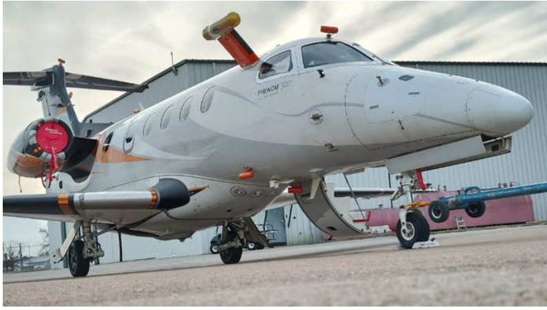
Fig. 1 Embraer Phenom 300 flight test bench: prototype aircraft with all modification for the SENS4ICE North America flight test campaign; credit Embraer.
