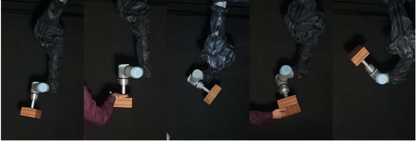
Fig. 5 Snapshots of satellite states at different times under free floating behavior with externally applied forces by human touch.
