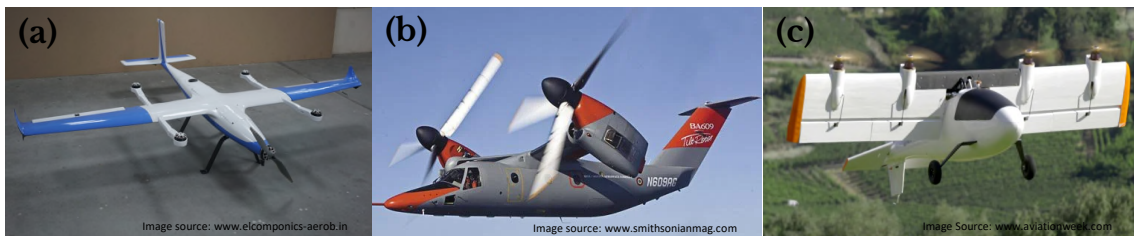
Fig. 1 Typical examples of (a) quadplane, (b) tilt-rotor and (c) tilt-wing aircraft
