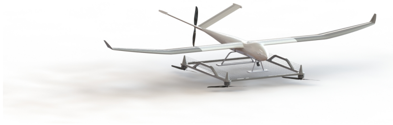
Fig. 2 Multirotor attached with fixed-wing UAV
