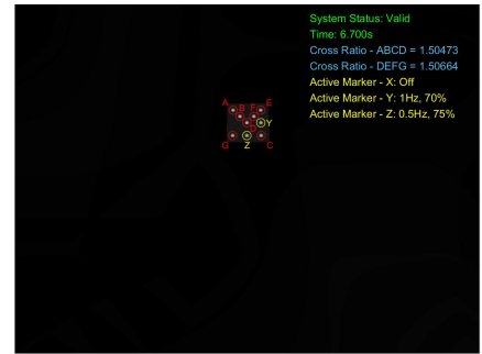
(e) In the image at 6.7s, the system has already tracked the active marker Z over 40 images. The active marker Z's frequency and duty cycle are calculated for the first time in the simulation (0.5Hz and 75%). Up until the current image, the landing pad is successfully recognized.
