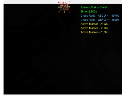
(b) In the image at 2.8s, the landing pad shows entirely for the first time, and the onboard system detects the landing pad successfully. In addition, the identification algorithm starts to track the status of each subsequent image from this image.
