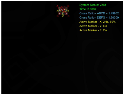
(c) In the image at 3.8s, the system has already tracked the active marker X over 11 images. The active marker X's frequency and duty cycle are calculated for the first time in the simulation (2Hz and 60%).
