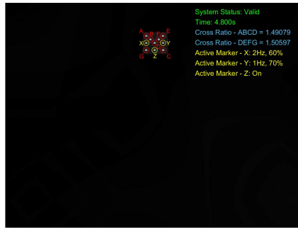
(d) In the image at 4.8s, the system has already tracked the active marker Y over 21 images. The active marker Z's frequency and duty cycle are calculated for the first time in the simulation (1.0Hz and 70%).
