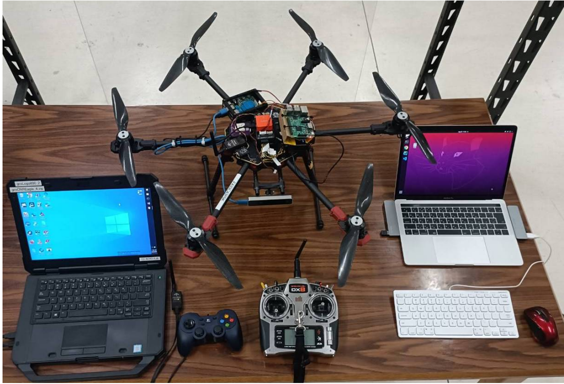
Fig. 6. The devices used for the flight test. From left to right: Ground Control Station (GCS) laptop, gaming controller connected to the GCS laptop, drone, radio controller for the safety pilot, and Linux laptop.
