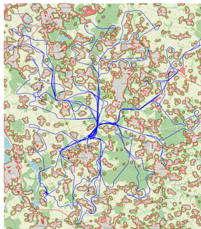
Fig. 6 Clustering and path planning results of one depot (blue lines). In contrast to solely clustering results the paths are smoothed and approved internally. The boundary of the operational volume is depicted in red, orange and green.
