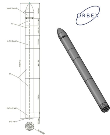
Fig. 1: Launch vehicle considered for Ascent scenario
