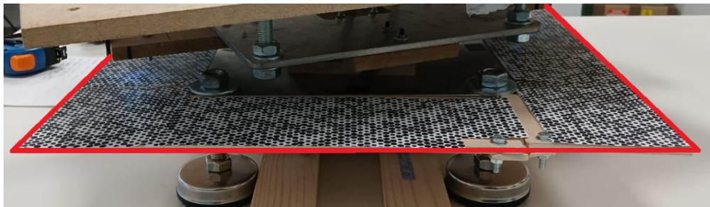
Fig. 7: Surface for optical flow detection on the TRACTOR-Beam platform.
